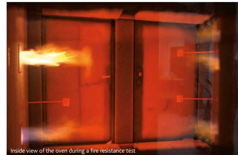
Inside view of the oven during a fire resistance test
